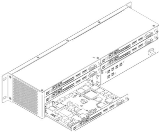
FIG. 2 Installing Cards
